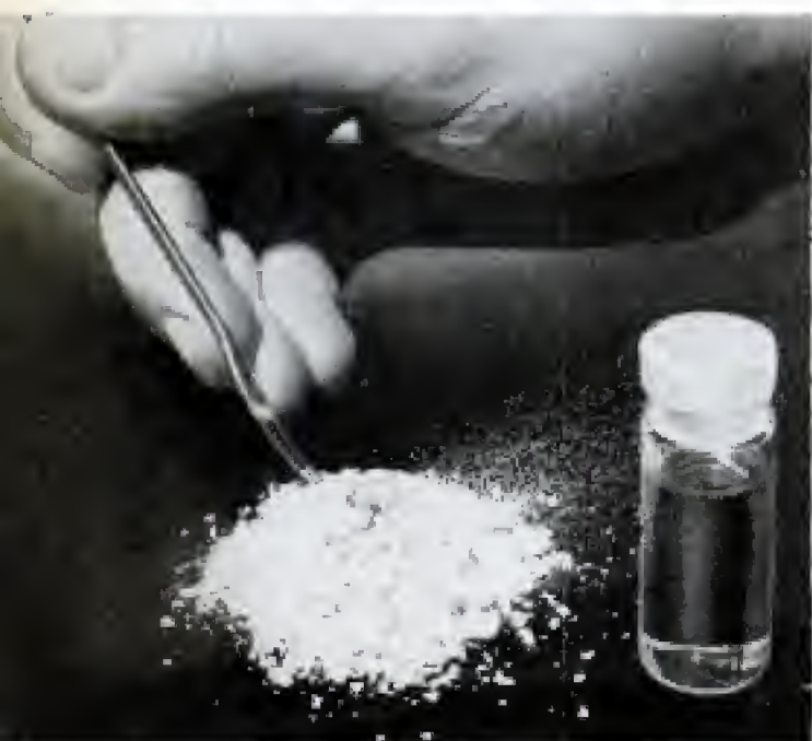
Slight irradiation causes a rubber band to crack and lose its elasticity (above), while two hours' exposure to gamma rays changes acrylonitrile from a liquid to a dry popcornlike polymer (below)
